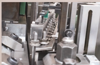
RP12 - Flat die thread rolling machine: 3 punch introduction system
