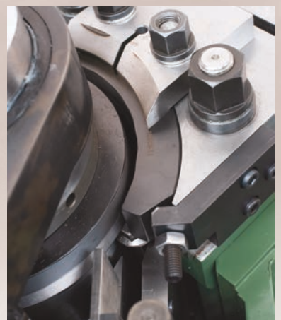
RP12 - Flat die thread rolling machine: 3 punch introduction system
