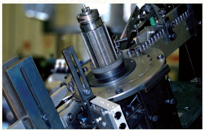
TLM washer/bushing loading machines are automatic assembly systems composed of 150/200/300 mm diameter carousels to allow for loading of micro-washers up to a washer diameter of 60 mm. The mechanics of these units are managed electronically via PLC with logics which ensures the total absence of production waste.
