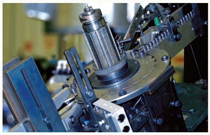
TLM Washer Loaders are automatic assembly systems composed of 150/200/300 mm diameter carousels to allow for assembling micro-washers up to a washer diameter of 60 mm. The mechanics of these units are managed electronically via PLC with logics which ensures the total absence of production waste.
