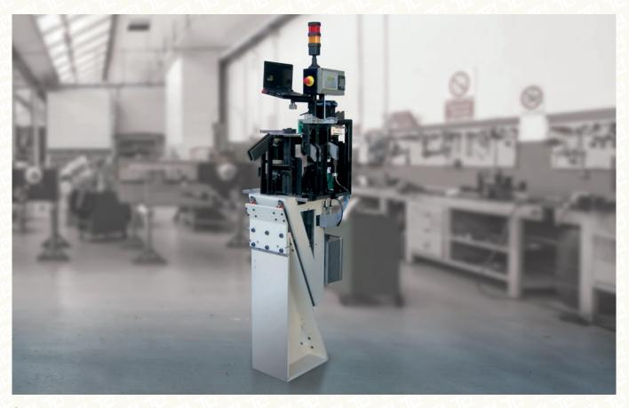
Sorting carousel, suitable for insertion in the production line for assembling washer screws and threaded screws, and able to carry out crack checks on hexagons, flanges and stems; check for crooked parts, with the possibility to scrap the faulty part.
