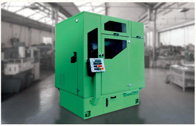
The chamfering machines can work at the highest production speeds with a careful fastening of the workpieces to prevent its rotation during the working. The machine can be delivered separately or coupled with a rolling machine and it is assembled
