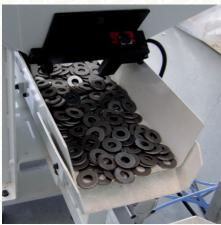
Consists of a loading hopper and a rising column on which a loading pallet is mounted. The latter, powered by the vibrating hopper – once the screws or washers have been loaded – rises along the column and unloads them directly into the rolling machine (threading machine) vibro-feeder. This system allows for reduced dimensions and loading spaces and for work cycle automation.
