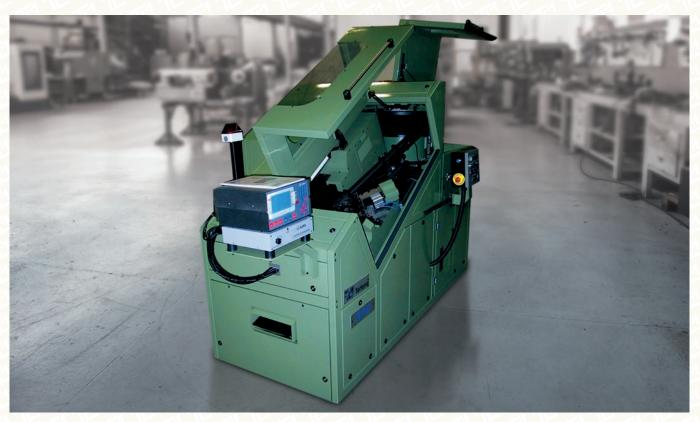
**1 punch machines**Single feeder machines have a feeder punch fixed to the punch holder, in turn installed on the single feeder runner whose kinematics and movement make the punch push and feed the
