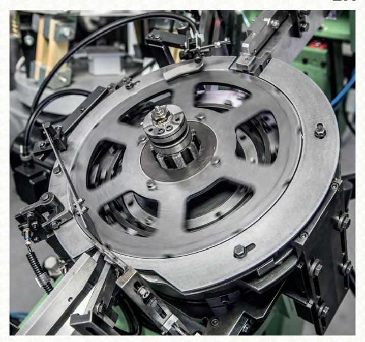
TLM's Bushing Loaders are automatic assembly systems designed on bushing shape and on customers' production needs.
